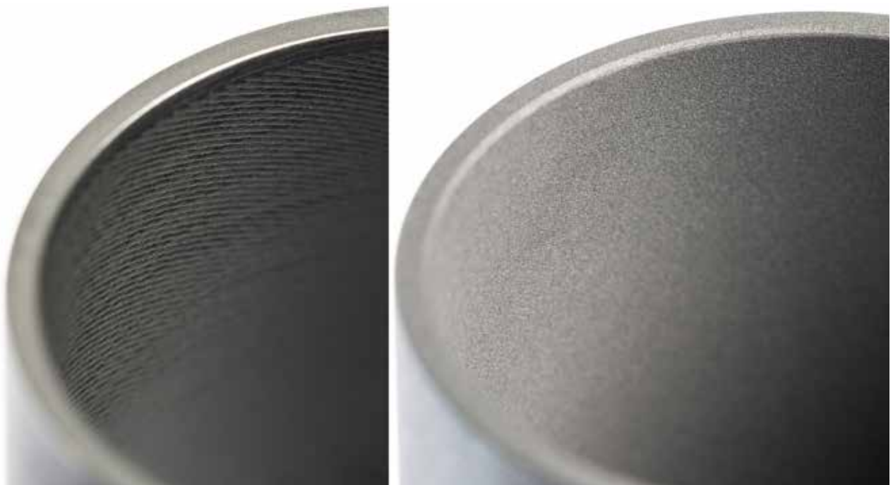
A close look reveals a significant improvement in surface finish. On the left, machined with carbide; on the right, with PCD.
