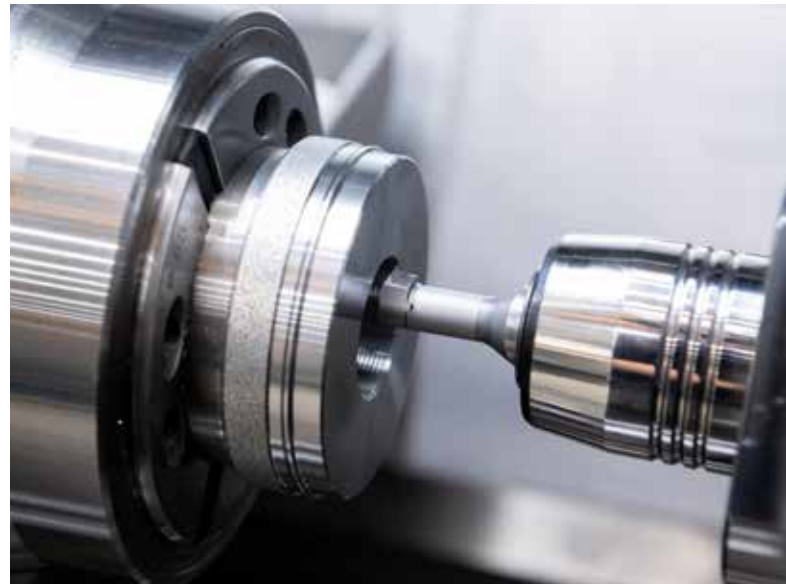
Internal threads in G30 carbide: The turning process, developed in collaboration with HORN, enables reliable thread production.
