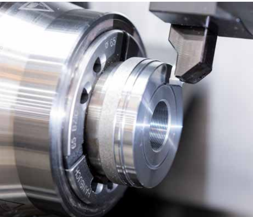
Axial groove in G30 cemented carbide: a particularly demanding machining operation that is carried out reliably at Linhardt Tec.Point.
