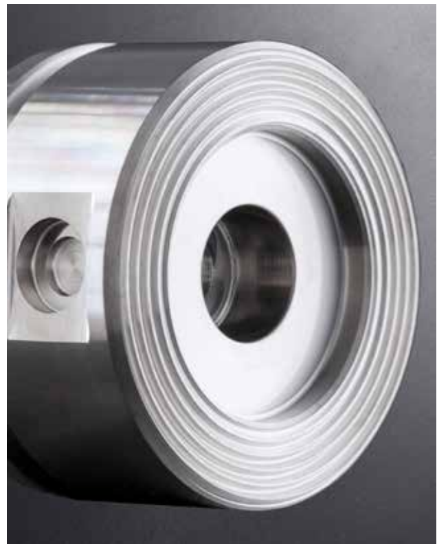
The use of CVD-coated tool systems enables complex contours to be machined in fully sintered cemented carbide.
