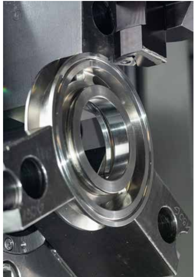
The System 315 handles axial grooving of O-ring grooves.
