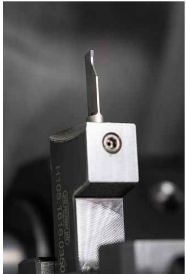
Parting off with a 1 mm (0.039") cutting width: HORN uses the Supermini system as the baseline for its designs.
