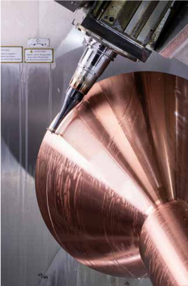
The tool mills several hundred metres of coolant slots into the combustion chamber.
