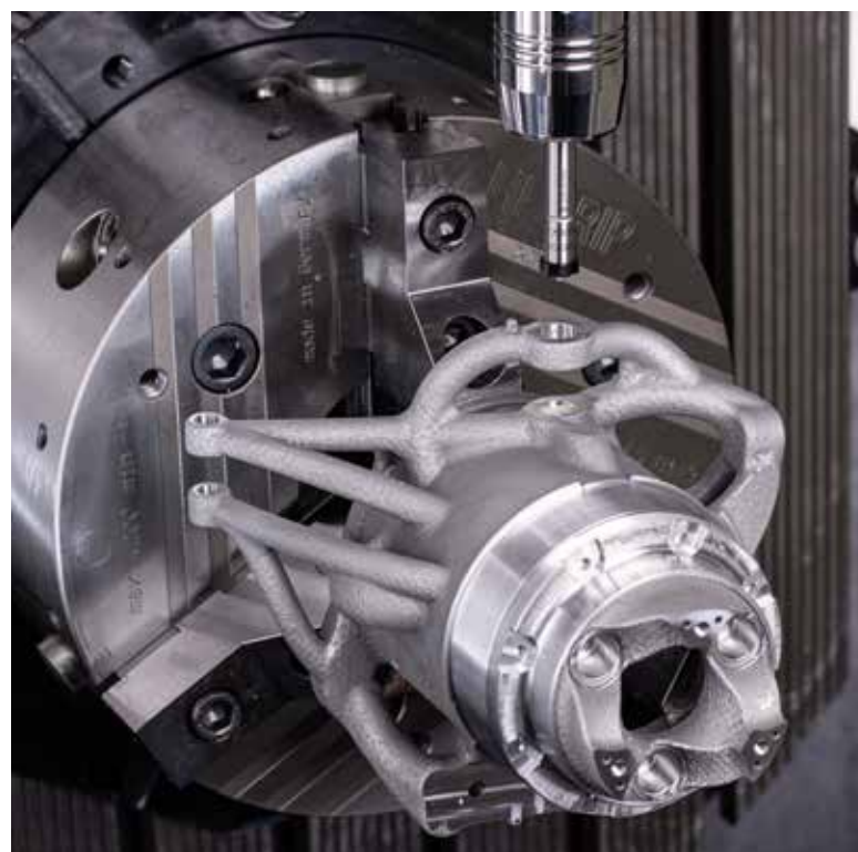
HORN's DR reaming system is used for reaming the fits.
