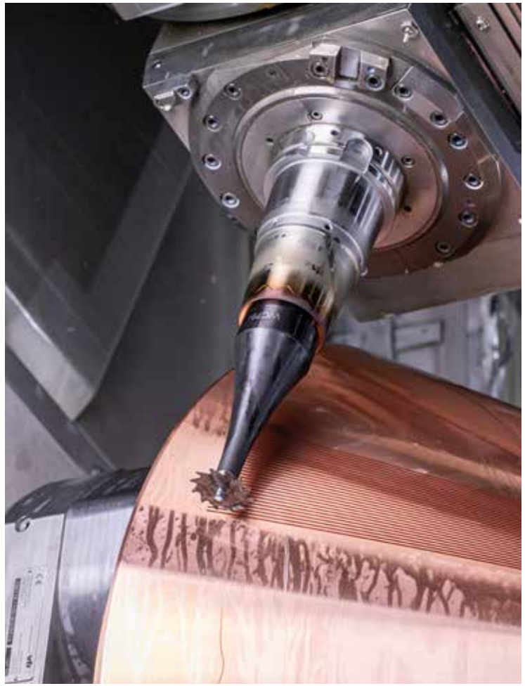
The solid steel tool holder is a finely balanced shrink-fit variety. This ensures low-vibration machining, despite the long overhang.
