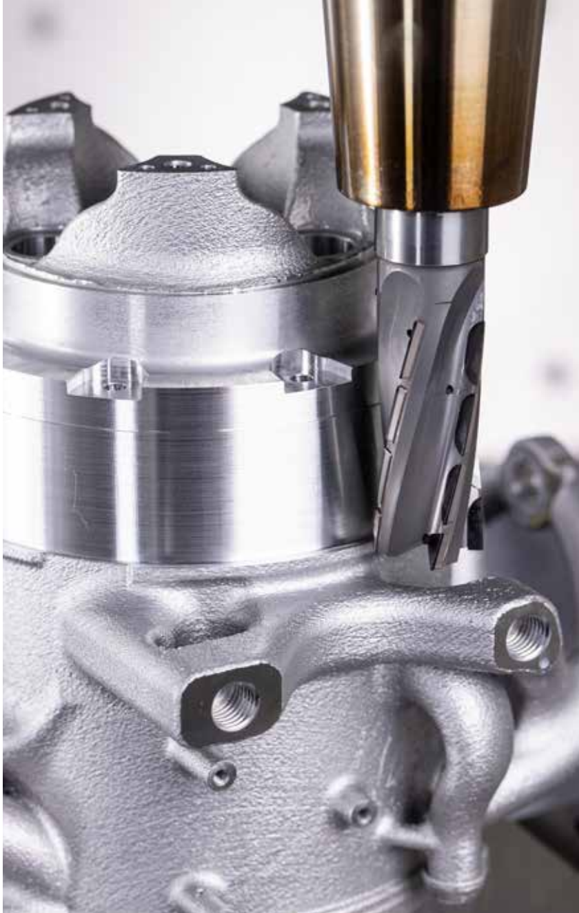
The HORN PCD milling system was also used.
