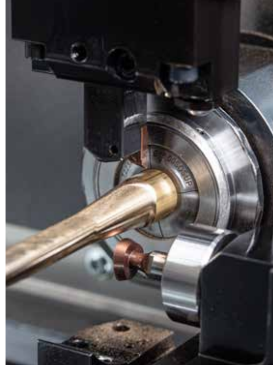
Left: High speed whirl milling (turn whirl milling) is a highly productive process for manufacturing bone screw threads. Middle: Eccentric turning enables highly productive manufacture of non-round external contours. Right: Polygon turning offers the possibility of producing non-round contours on lathes.
