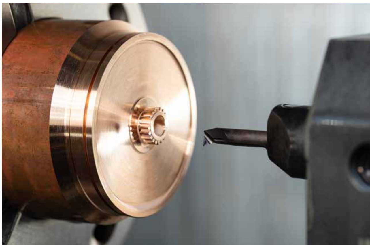
Boring the inside of the central hole with a HORN Supermini.
