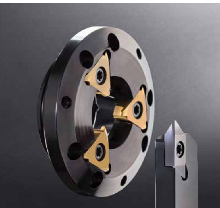
High-speed whirling enables continuous cutting through concurrent turning.
