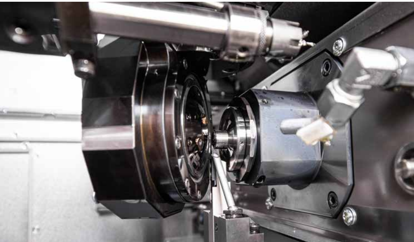
The carbide grade IG35 is used for machining titanium alloys.
