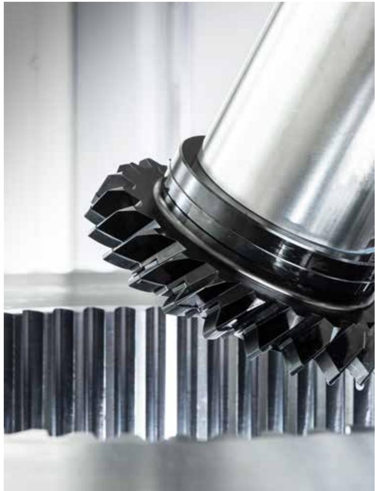
For larger modules, HORN also offers gear skiving systems with indexable inserts.
