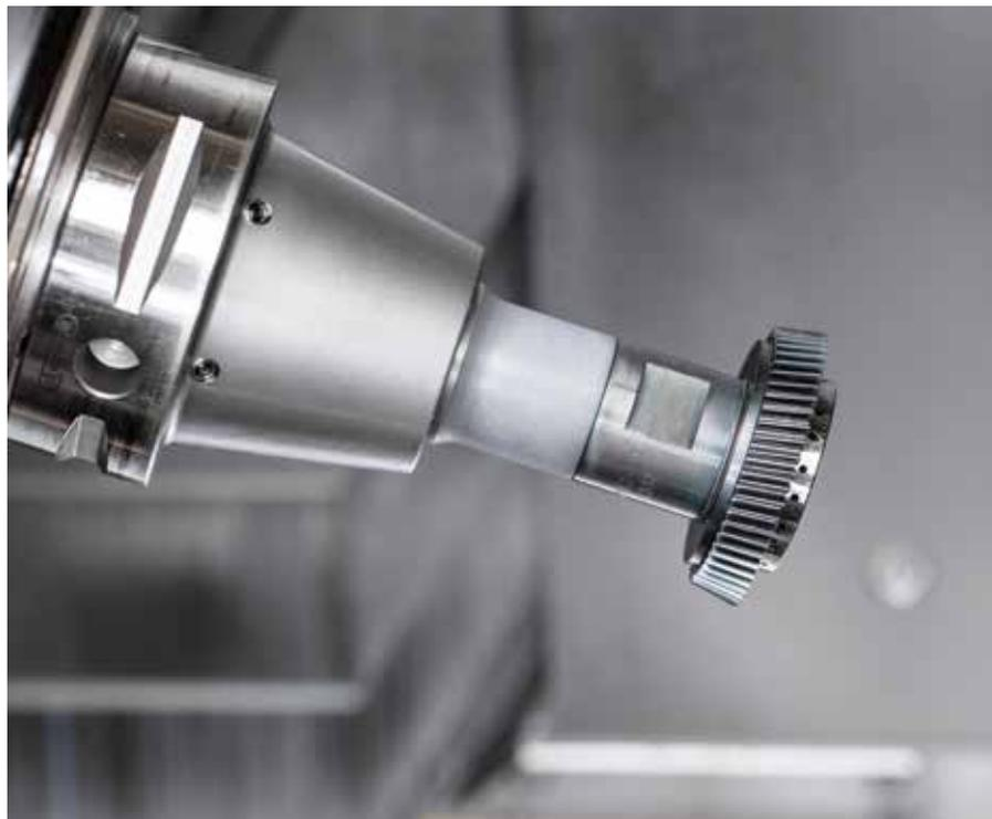
More than 40 variants of the precision tools are in use at Neugart for producing gears from module 0.5 to 2.
