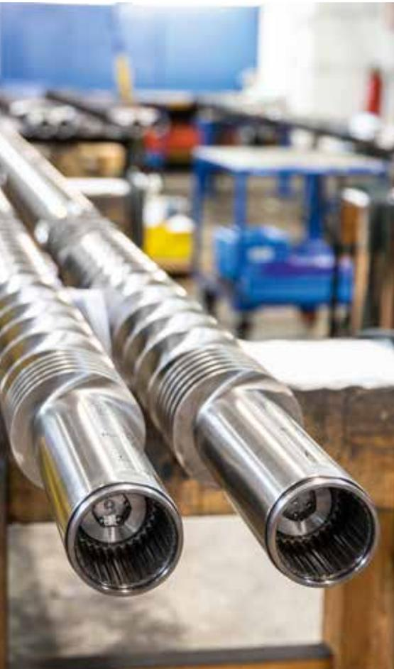
Modular design: two extruder screws under construction. The sleeves are visible at the front.
