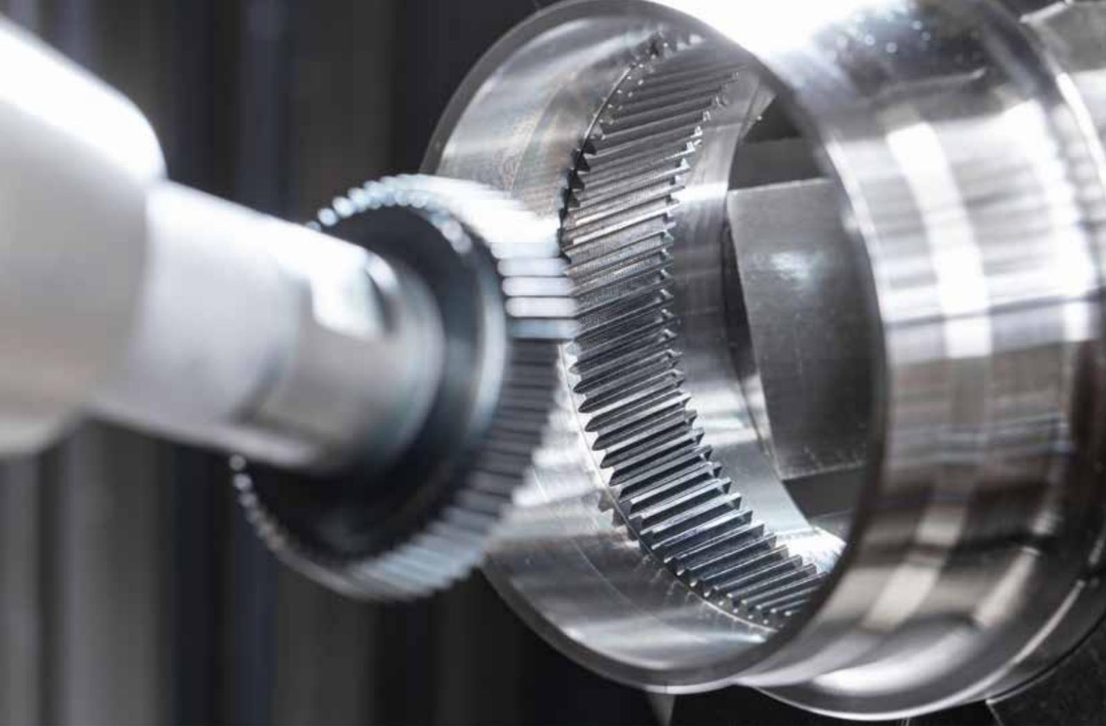
For gear skiving, Neugart relies on tool systems from HORN.
