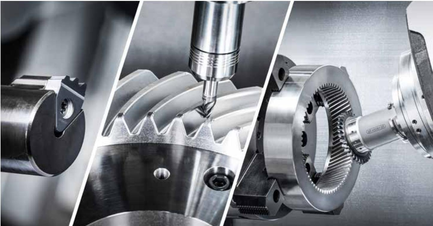
The cooperation is centred on gear broaching, gear milling and gear skiving.
