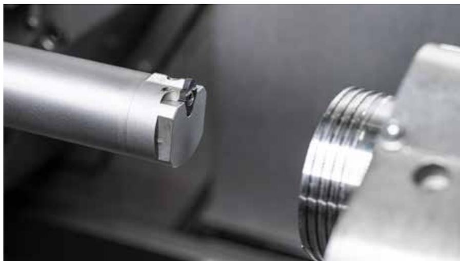
HORN relies on the 117 system for broaching the spline.
