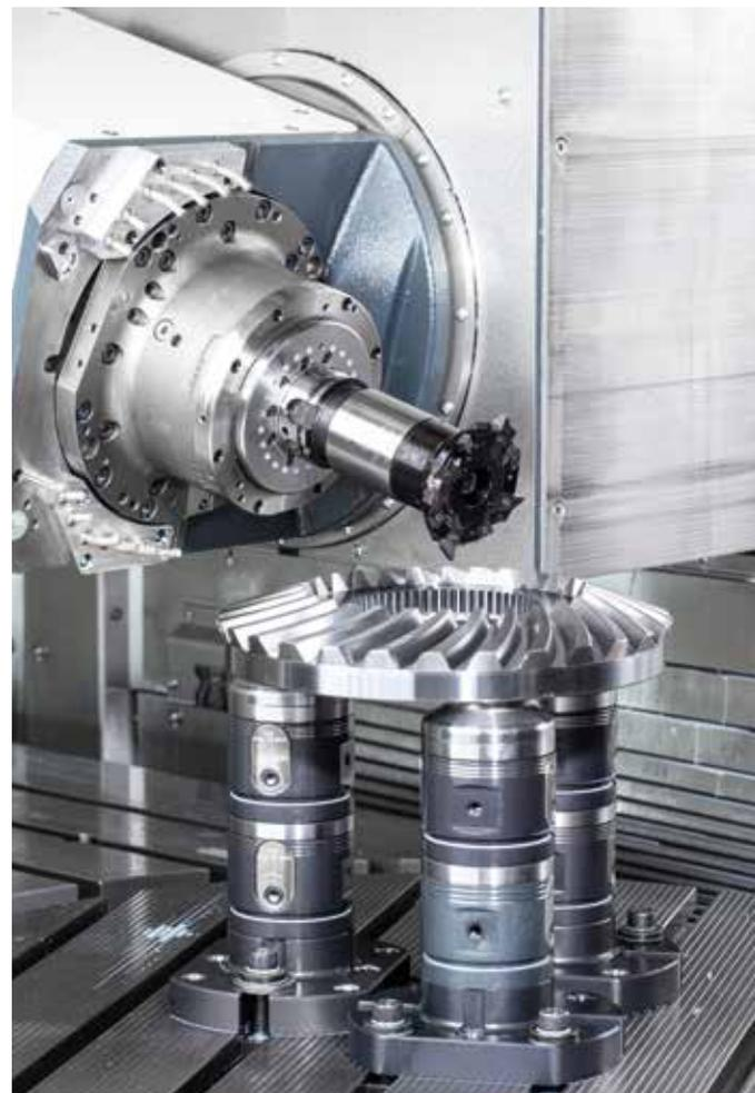
HORN developed the M279 milling system for economical roughing of cyclo-palloid gears.
