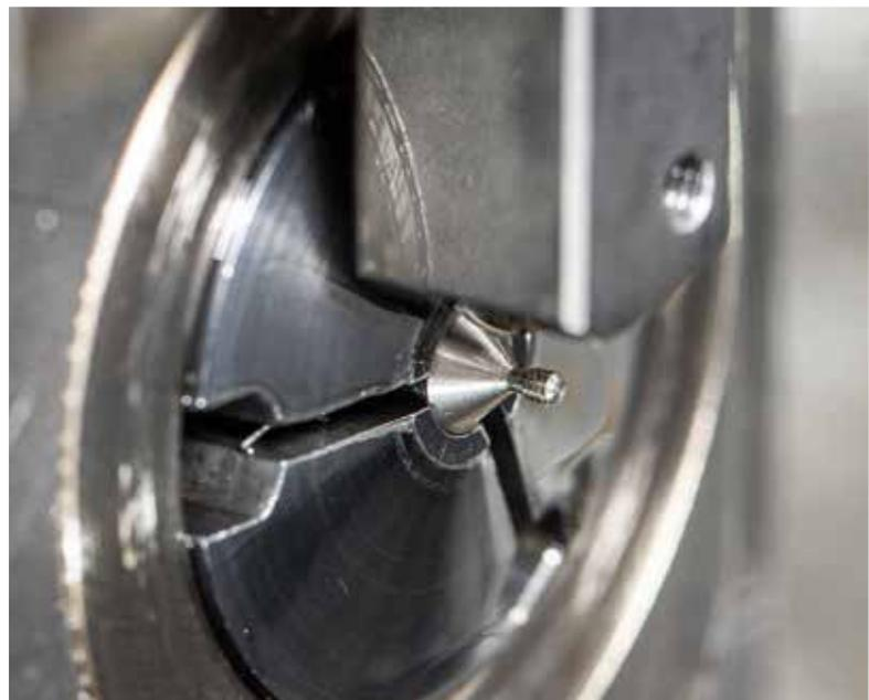
Turning the M1.6 x 0.35 thread with the S274 system.
