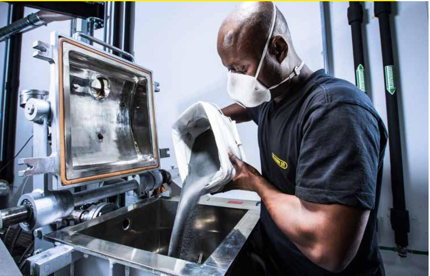
The manufacturing process for an insert starts with mixing and preparing carbide alloys in powder form.
