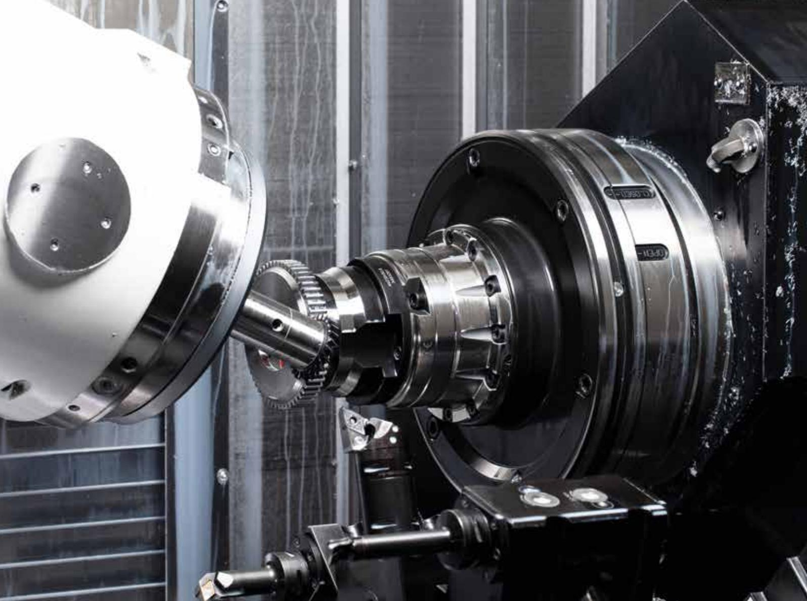
Prior to the introduction of the gear skiving process, the components were being manufactured with conventional cutting tools. "We were in the process of reorganising the production of our families of gears", explains Pascal Moulènes. With the help of the new technology, Moulènes was able to optimise the production processes because fewer set-up operations were required and he also managed to eliminate the idle time between work
