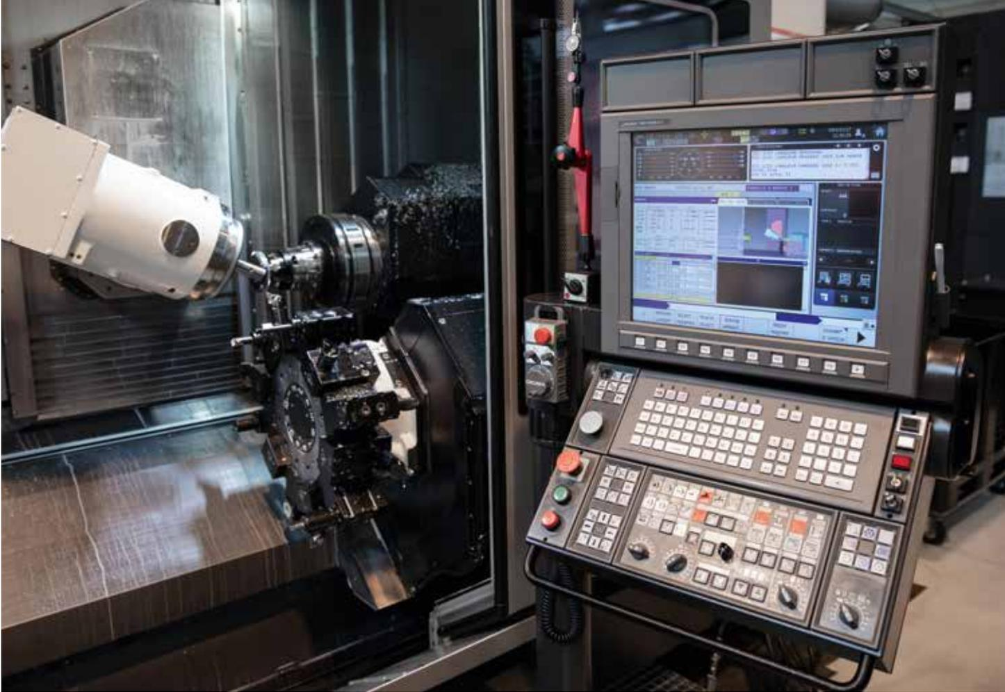
Gear skiving can be easily programmed on modern CNC production centres.
