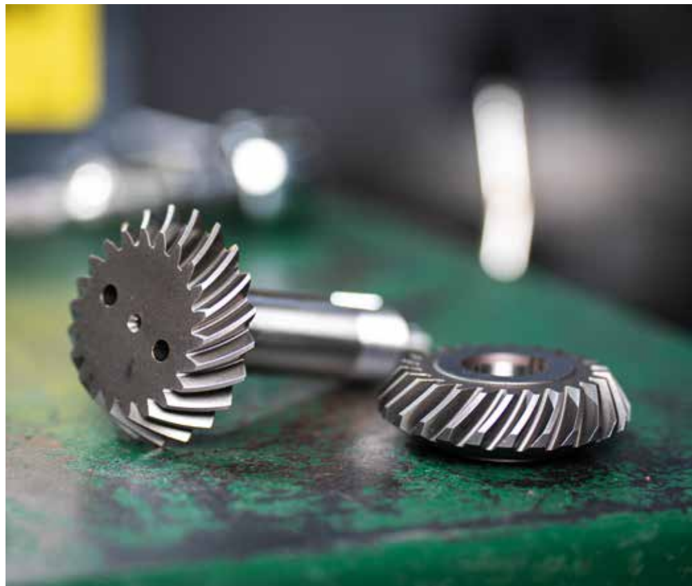
60-degree PTO bevel gear set for a military land vehicle.
