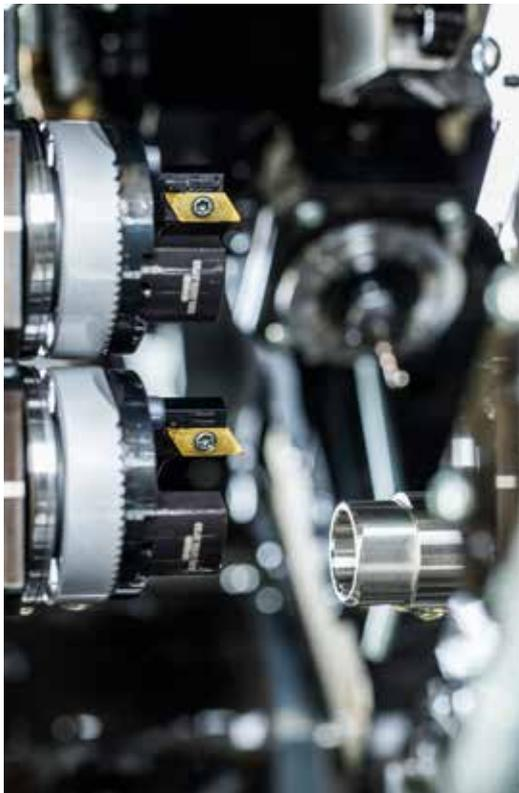
HORN has developed tools for the polygon turning process to manufacture non-circular contours.
