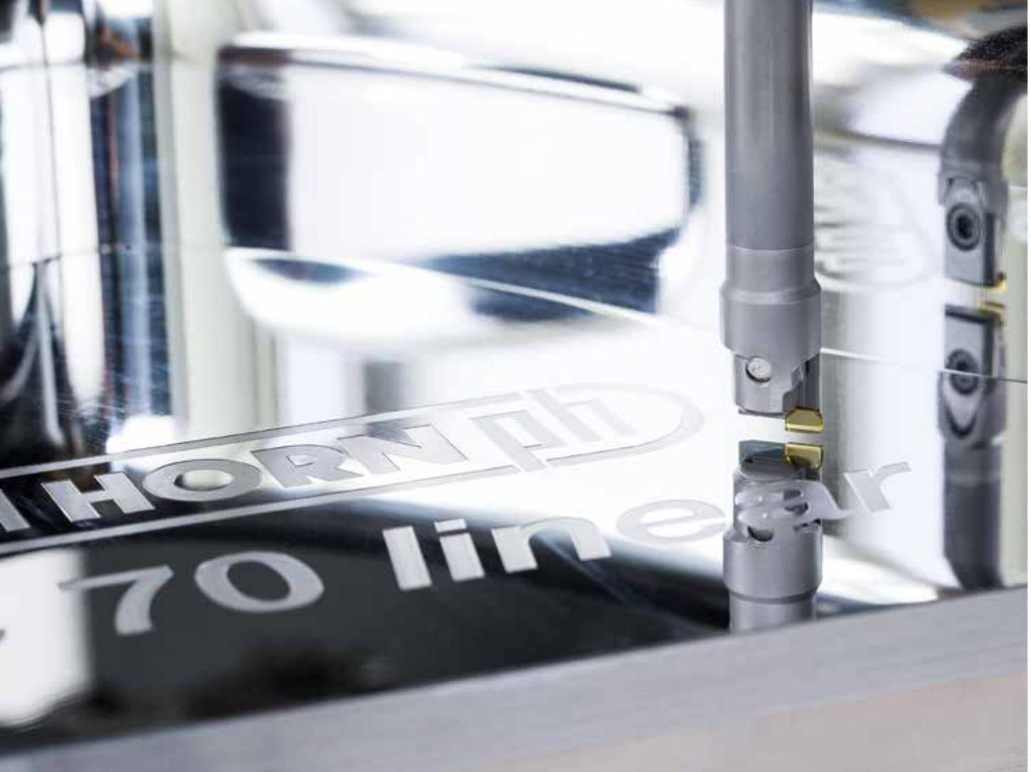
Mirror finish over the entire surface. HORN and DMG MORI use a sine wave to demonstrate their expertise in brilliant-finish machining of aluminium.
