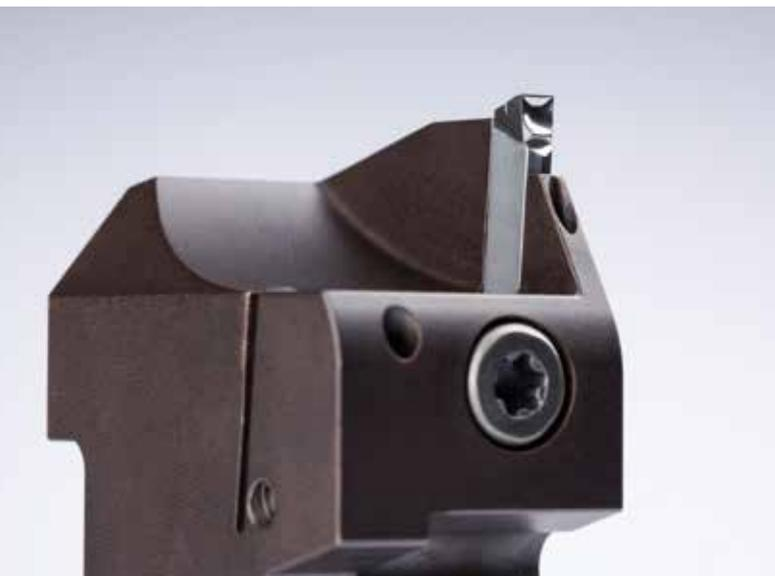
The polished WA chipbreaker geometry enabled problems of long chips and built-up edges during aluminium machining to be resolved.
