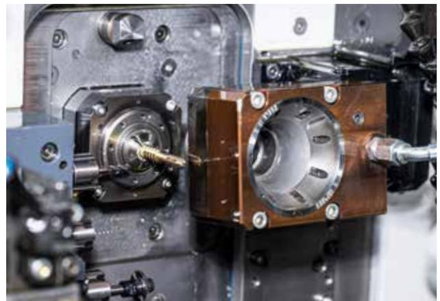
Jet whirling has reduced the machining time for worm threads by half, raised quality and ensured an increase in tool life.
