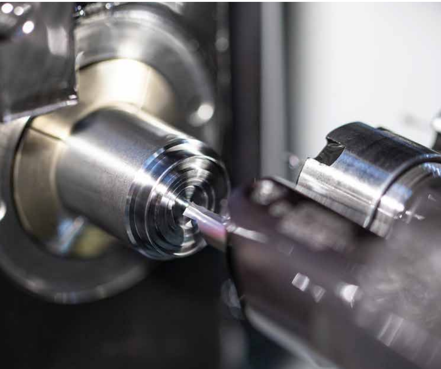
Axial grooving of the valve cover with the Supermini 105.
