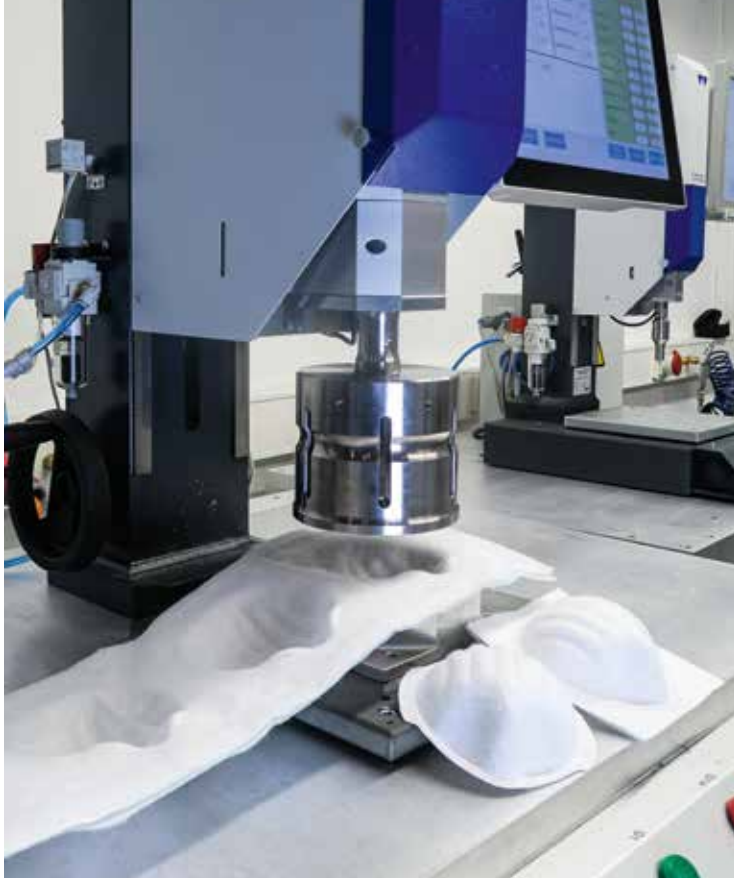
The ultrasonic welding process from Weber Ultrasonics is used to produce surgical masks.
