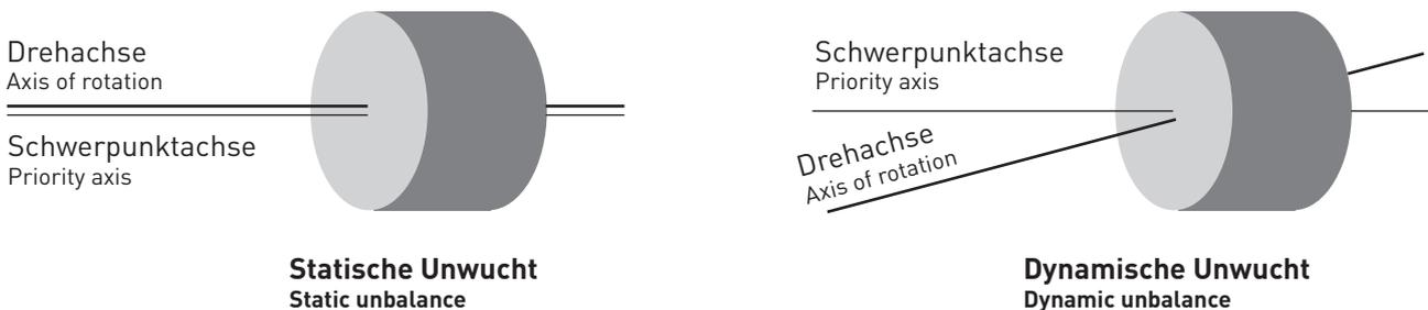
Rotating Unbalance is the uneven distribution of mass around an axis of rotation. Unbalance is caused when the centre of mass (inertia axis) is out of alignment with the centre of rotation (geometric axis)....
